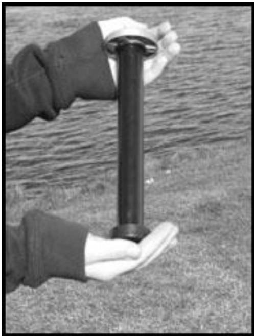
Fig. 4 – Remove or shorten center post for more stability.
