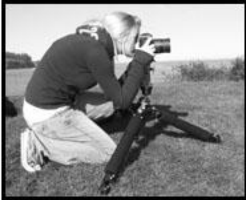
Fig. 2 – Tripod legs should be able to lay out nearly flat.
